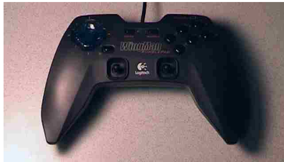
Figure 2.5: Logitech WingMan RumblePad controller used to control the robot arm and user interface in the experiment.
